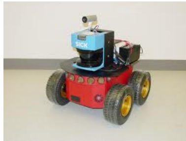
Figure 2. Picture of the mobile robot Pioneer 3AT used in this work. The range sensor laser is mounted on the vehicle.
