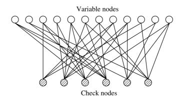
Figure 4. Bipartite graph corresponding to an irregular parity check matrix.
