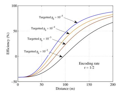
Targeted BER is the parameter that indicates the reception quality of the signal. The cooperative MIMO communication used in this paper is simulated with a fixed value of targeted BER. Figure 11 shows that the change in targeted BER changes the efficiency of cooperative communication over SISO transmission. Result shows that the cooperative communication is more energy efficient than SISO transmission in smaller targeted BER.
