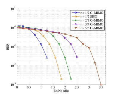
The same BER analysis is taken in Figure 10 in a Nakagami fading channel scenario. The result shows that the decrease in Nakagami coefficient m degrades the error performance.
