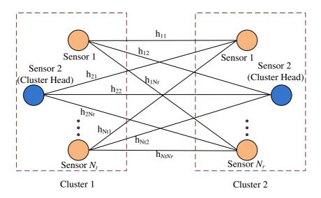
Figure 1. System model for cluster to cluster communication in wireless sensor network.
