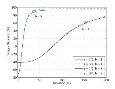
Figure 8. Energy efficiency for different constellation sizes.
