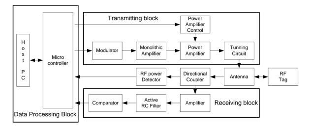
Figure 2. Block diagram of UHF RFID reader.
