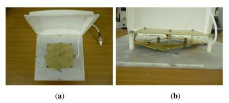
Figure 8. UHF RFID antenna: (a) top view and (b) side view.
