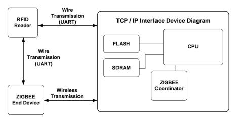
Figure 1. System configuration.
