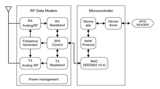
Figure 5. Prototype of ZigBee End-device.
