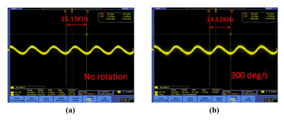
Figure 8. Sensitivity evaluation of the fabricated SAW gyroscope.
