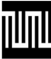
The low value of electromechanical coupling for ST-cut quartz causes high losses in mismatch of its input impedance up to 50  $\Omega$ . In order to minimize the losses an operation mode of IDTs has been set to match 50  $\Omega$  impedance for 74 MHz frequency. Figure 13 presents the way the transducer has been matched.
