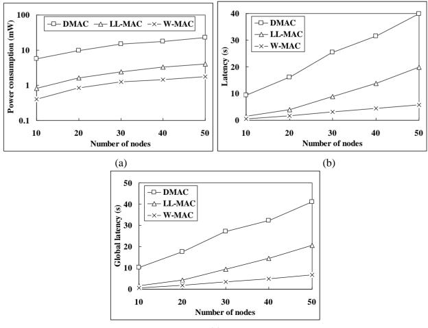
Figure 8. Protocols comparison: (a) power consumption; (b) latency and (c) global latency.
