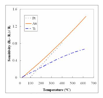
Figure 2. The linearity comparison of sensing materials [19,20].
