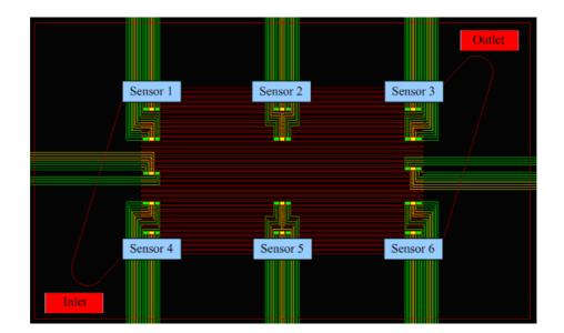
Figure 7. Distribution of micro temperature sensors during calibration.
