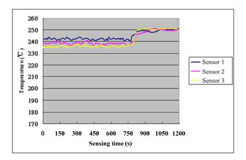
**Figure 8.** Temperature distribution of micro sensors  $1 \sim 3$  insider the reformer.
