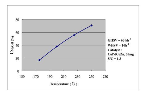
Figure 6. Relative curve of conversion and temperature under the SRM reaction.
