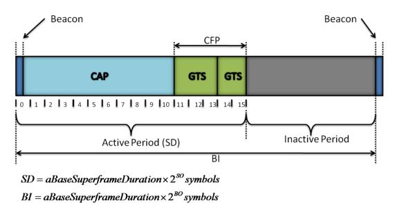
Figure 2. Example of the superframe structure of IEEE 802.15.4.
