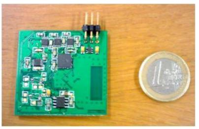
Figure 11. Wireless sensor node prototype board.
