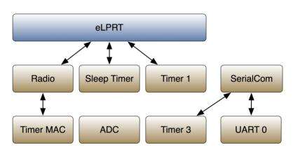
Figure 12. System software modules.
