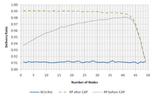
For both cases, as the number of nodes approaches the capacity of the network, the space available for retransmissions in the superframe decreases and, consequently, the delivery ratio approaches the value without retransmissions.
