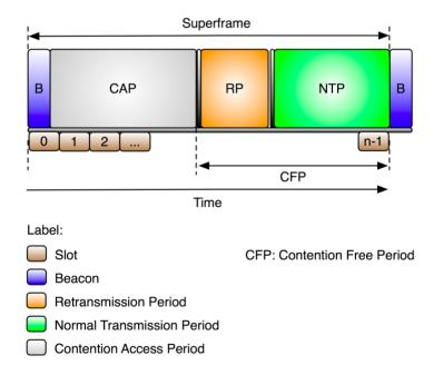
Figure 3. Superframe structure of the eLPRT protocol.
