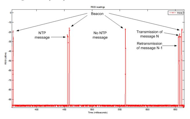
Figure 14. Example of operation of the contention-free retransmission mechanism.
