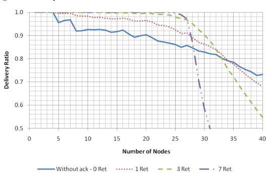
Figure 4. Delivery ratio for the unslotted CSMA/CA scheme with error-free channel.
