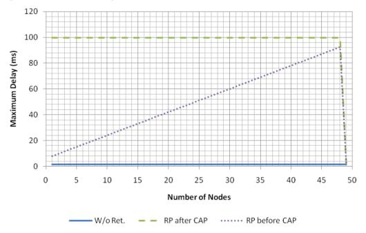
**Figure 9.** Maximum delay of eLPRT with  $BER_{bad} = 10^{-2}$  (data) and  $10^{-4}$  (beacon).
