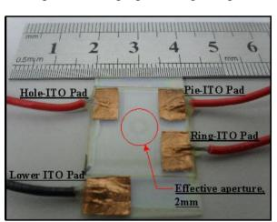
Figure 5. The photo of the proposed ring-and-pie DFLC lens.
