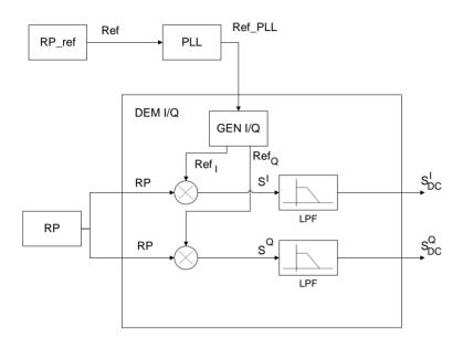
Figure 11. Signal treatment block.
