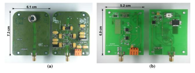
Figure 13. (a) Receiver PCB; (b) Emitter PCB.
