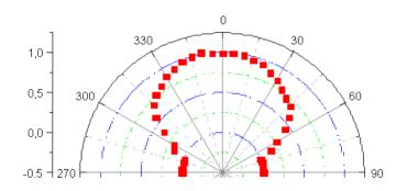
Figure 6. Reception pattern of the receiver device.
