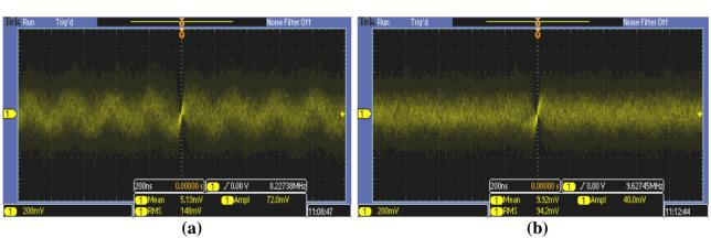
**Figure 10.** Signals in the output of the receiver: (a) Best case:  $(2.5 \text{ m}, 0^\circ)$ ; (b) Worst case:  $(3.5 \text{ m}, 45^\circ)$ .
