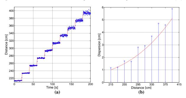
Figure 15. (a) Distance measurements using one receiver; (b) Dispersion for each distance  $(2\sigma)$ .
