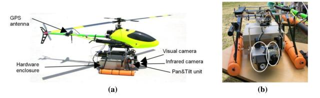
**Figure 4.** Diagram of the proposed forest-fire measurement system.
