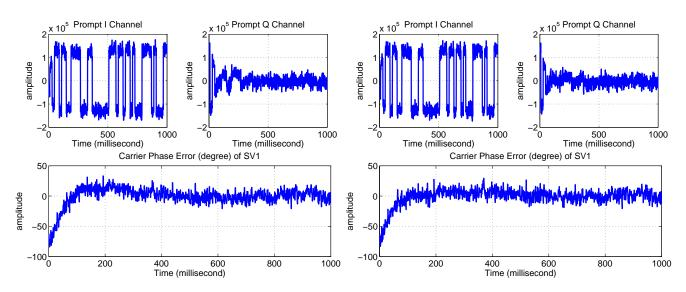
Both systems are tested on a NORDNAV R25 software GPS receiver. This receiver collects, down-converts and samples the GPS data by the front end, so that the collected GPS data can be post-processed repeatedly using different tracking-loop filter orders. The results are shown in Figure 12.
