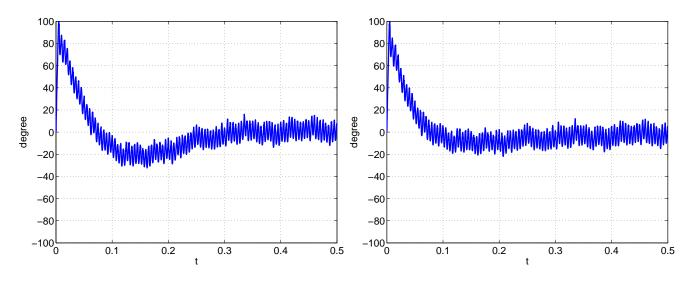
Figure 11. Phase error of Simulink simulation. Left: linear design. Right: nonlinear design.
