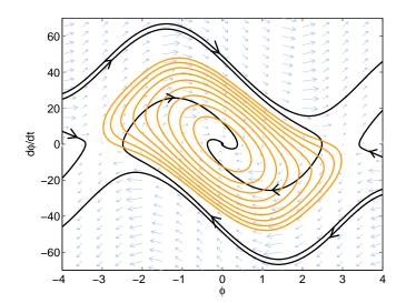
Figure 9. Local Lyapunov level sets of the original PLL system.
