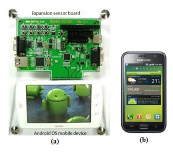
The ECG monitoring system was developed and tested on an Android<sup>™</sup> mobile platform development kit [10] as shown in Figure 6(a), running an ARM processor (S5PC100X—ARM-CORTEX A8). This development kit comes with a sensor expansion board and an Android<sup>™</sup>-based smart phone-alike mobile device. Through the serial port, the sensor expansion board is able to connect
