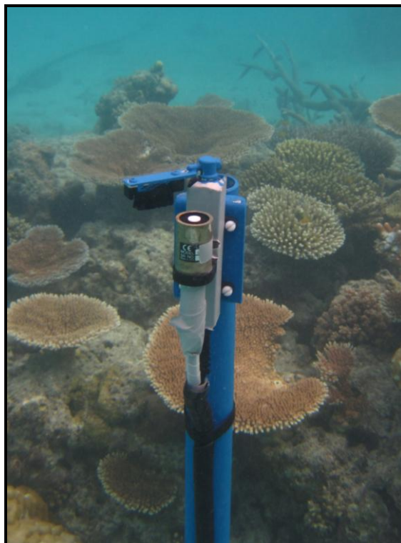
Figure 5. Light Meter installed showing the wiper system in-place.
