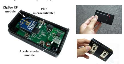
**Figure 1.** The prototype of the wearable motion detector.
