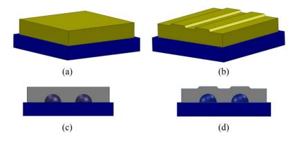
The indenters were applied vertically on the skin covers and to the center of the four sensors on the Tactologic sensor pad to obtain their force profile. Figure 4 shows the cross-section of the indentation applied to the skin covers on the sensor pad.
