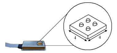
The sensing technology of the sensors is piezoresistive and the size of total active area is  $4 \text{ mm} \times 4 \text{ mm}$  with 5 mN/bit normal and 2 mN/bit shear sensitivity. This sensor can detect and measure the force values of the contact in both normal and tangential directions. It has been shown that the three-dimensional signals generated by this sensor provide the possibility for basic six Degree Of Freedom (DOF) spatial-temporal tactile measurements on arbitrary objects.
