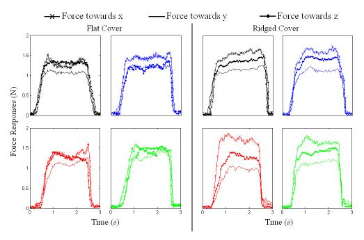
**Figure 8.** Sample runs of the experiment for flat and ridged skin covers. The responses correspond to the resultant forces from the four sensors of the tactile sensor array.
