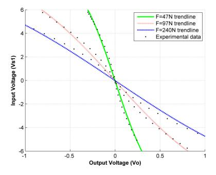
Despite the fact that the coefficient of determination remained high for all sensors under study (exhibiting an average value of  $R^2 = 0.991$ ), it is clear that Equations (8) and (15) require some changes in order to provide a better fit. So far we have not found a suitable and simple curve for modeling sensor behavior under such driving conditions.
