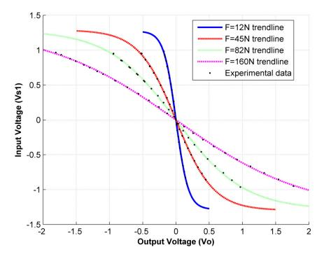
Parameters k and q were set to adjust independently for every applied force, however, the independent fitting processes returned values of k that remained almost constant, regardless of the exerted force, F, whereas q was shown to be hyperbolically dependent on the exerted force. In other words, 1/q is a linear function of F. Figure 4 shows the variation of k and 1/q for different applied forces within the 0 N–250 N range resulting from independent fitting processes.
