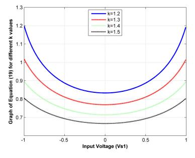
Equation (19) is a measure of how the sensor conductance is affected by changes in the input voltage. The higher k is for a given sensor, the flatter the lines in Figure 6. This can be understood as a less-noticeable amplitude nonlinearity in the sensor.
