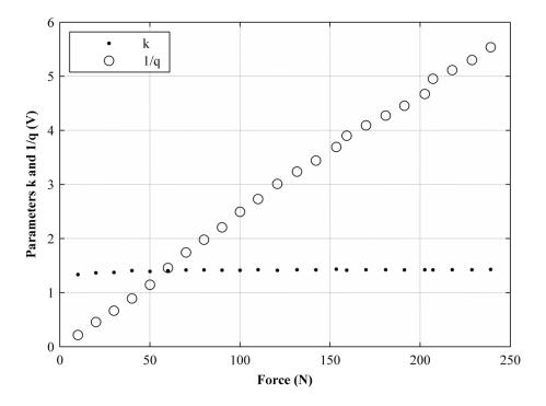
With the aim of demonstrating that Equation (11) is an approximate expression for fitting the data points from Figure 3, the 1/q curve from Figure 4 is taken and represented as linearly dependent on the applied force:
