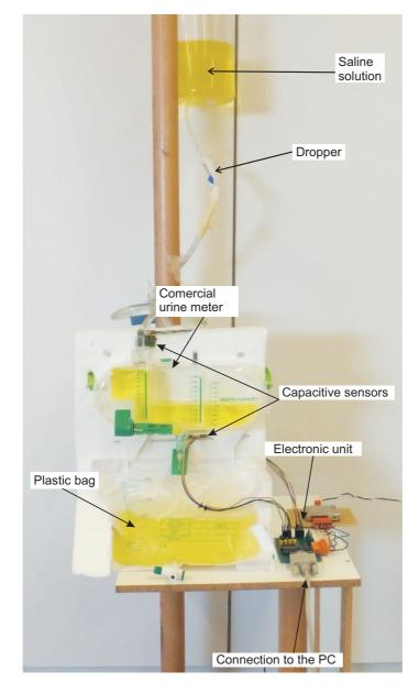
Figure 7. Prototype of our device built with a commercial urine meter.
