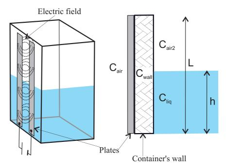
In our problem, on one side of the capacitor, the dielectric will be the air. On the other side, we first have the wall of the container, and then air, or liquid, or a combination of both (see Figure 2). In this situation, it can be proved that the total capacitance of a multi-dielectric layer coplanar-plate capacitor can be calculated as the sum of four terms, each of them given by Equation (1) [21]:
