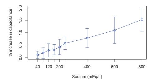
Although these tests were conducted with a container completely filled with liquid, as can be seen in Equation (6), for any height of the column of liquid a change in the concentration of sodium (and therefore on the dielectric properties of the liquid) will produce the same change in percentage in the measure of the capacitance for any height of the liquid column.
