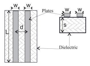
Figure 1. Coplanar-plate capacitor.
