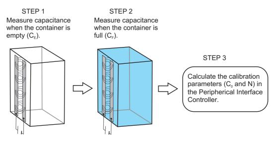
Then, we shall measure the capacitance when the container is completely full. Let us suppose that the measured capacitance is  $C_F$ . If the height of the liquid column at this moment is L then:
