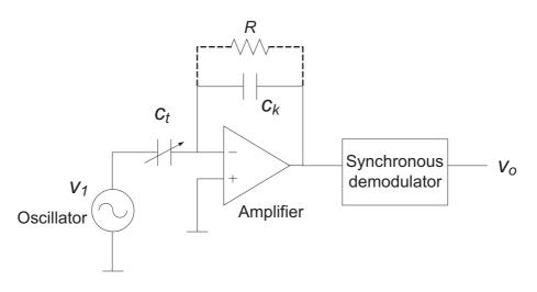
Figure 4. Measurement of the capacitance of the capacitive sensor.
