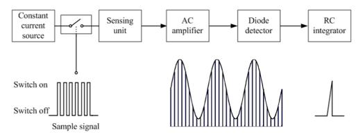
Figure 2. Description of how TDM works in the RIP module.
