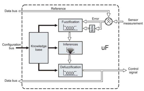
In a fuzzy controller the input measurement coming from the smart-sensor is subtracted from the reference set-point, then, the error between the desired value and the measured value is used as input for the fuzzy logic algorithm. In this case, the proposed uF is designed as 2-input 1-output system, the inputs are the error and its derivative which is a common practice in the design of fuzzy controllers [27]. The output corresponds to the control variable applied to the actuator.
