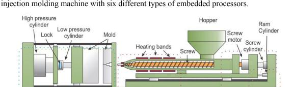
Figure 2. Embedded smart-sensor and controlling network architecture to control a plastic
