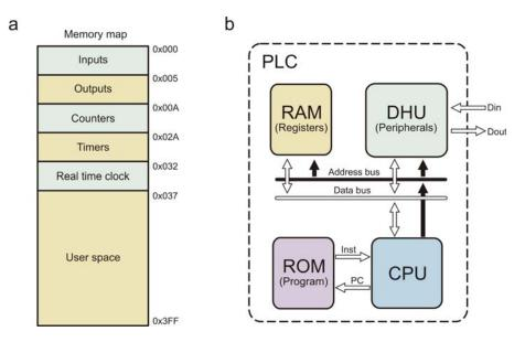
Figure 5. (a) PLC memory map. (b) PLC architecture.
