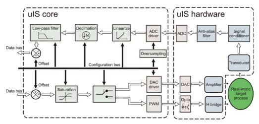
The uIS hardware receives the transducer signal, conditioned to an industrial standard of  $\pm 10$  V and filtered by an anti-alias filter; then, the ADC converts the analog signal to a digital number. The DAC is directly connected to a power amplifier, while the input PWM signals are optically isolated from the H-bridge.
