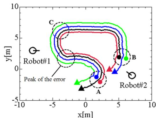
Figure 8(a) shows the effect of tracking mode and data association methods to the tracking error; GNN and conventional nearest neighbor (NN) [24] methods are applied for the data association. Tracking error is evaluated by the following root mean squared error (RMS):
