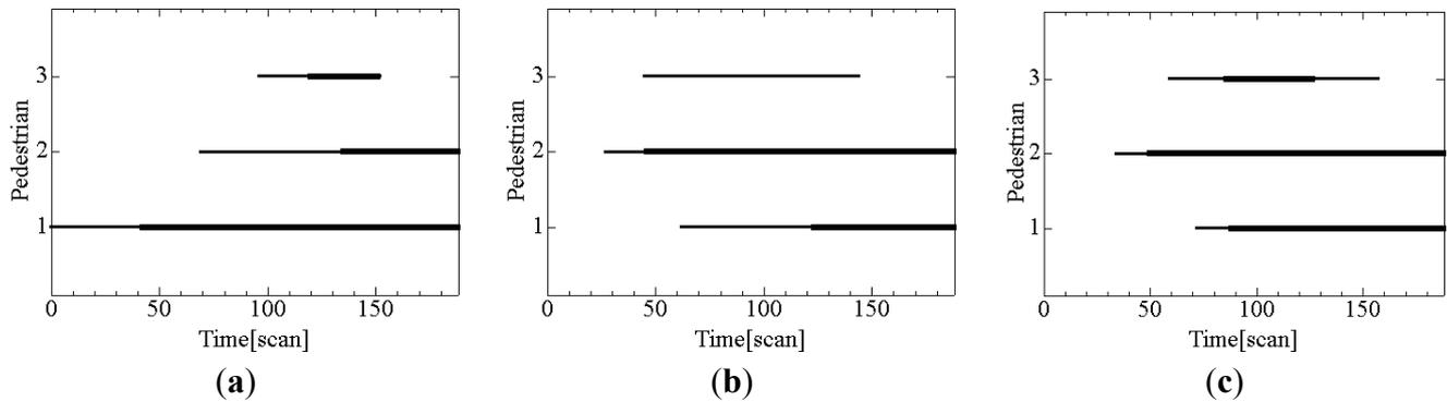
**Figure 14.** Duration of individual and cooperative tracking. The thin line indicates the time during which the pedestrian exits the sensing area of each robot. The bold line indicates the time during which the robot tracks pedestrians using the individual and cooperative tracking.
