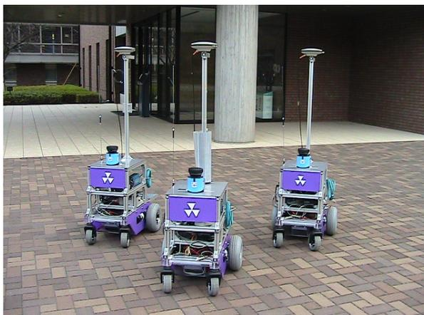
The robot is equipped with a single-layered LRS (Sick LMS100). The LRS captures laser scan images that are represented by a sequence of distance samples in a horizontal plane of 270 deg. The angular resolution of the LRS is 0.5 deg, and the number of distance samples is 541 in one scan image. The onboard computer is a Lenovo ThinkPad R500 with a 2.4 GHz Intel core 2 duo processor, and the operating system used is Microsoft Windows Vista. The sampling frequency of the sensors is 10 Hz.
