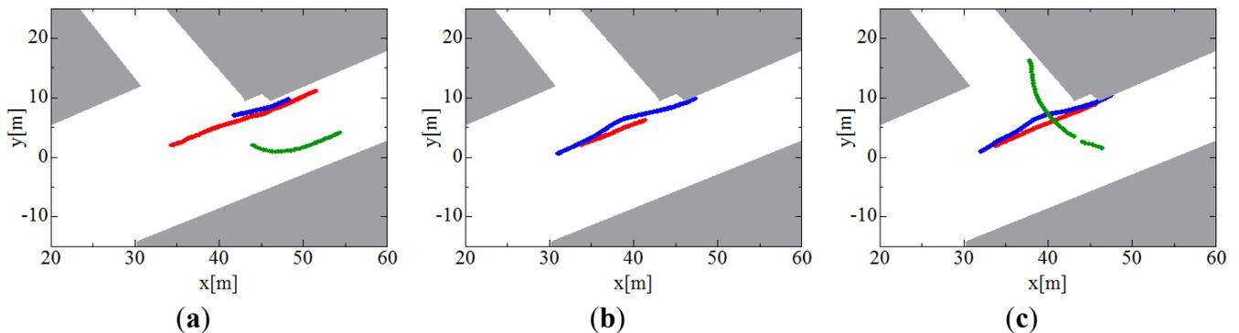
Figure 12 shows the tracks of three pedestrians estimated by individual and cooperative tracking; because the three robots share the tracking data with each other, all three robots can track the three pedestrians for an extended period.
