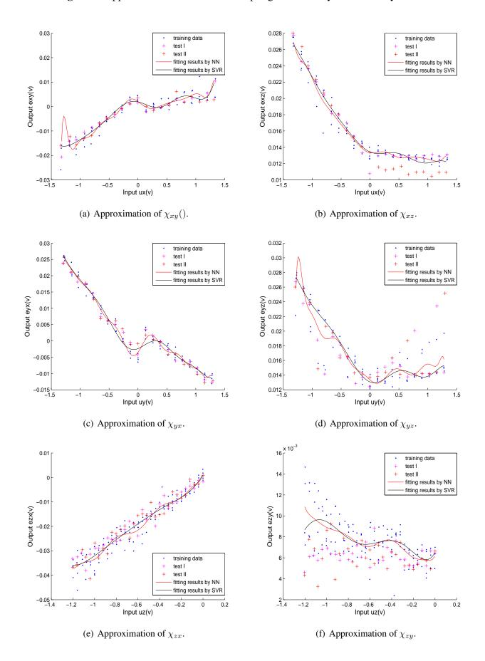
Figure 7. Approximation of corrected coupling functions by  $\epsilon$ -SVR vs. by RBF NN.
