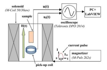
The frequency spectrum of the voltage pulse g(f) was calculated using the discrete Fourier transform function in LabView. For all CoFe samples the dependencies of the ME conversion coefficient on the frequency f at DC bias field  $H_{\rm m}$  and at fixed frequency f on the DC field H were also obtained by the standard method of harmonic field modulation (HFM) ( $\delta h = 1$  Oe, f = 100 Hz–300 kHz, bias field  $H_{\rm m} = 650$  Oe) [17].
