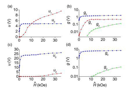
The growth of the oscillation amplitudes  $u_1$  and  $u_2$  with the increasing excitation pulse magnitude  $\hat{H}$ , even after the pulse amplitude  $u_0$  was saturated (see Figure 5), can be explained as follows. For the magnetic pulse of fixed duration, the increase of the magnitude  $\hat{H}$  results in the corresponding growth
