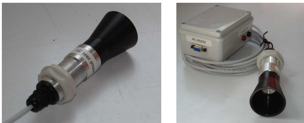
Figure 2. Ultrasonic sensor with ultrasonic transceiver built in the horn. The enclosure includes sensor electronics.
