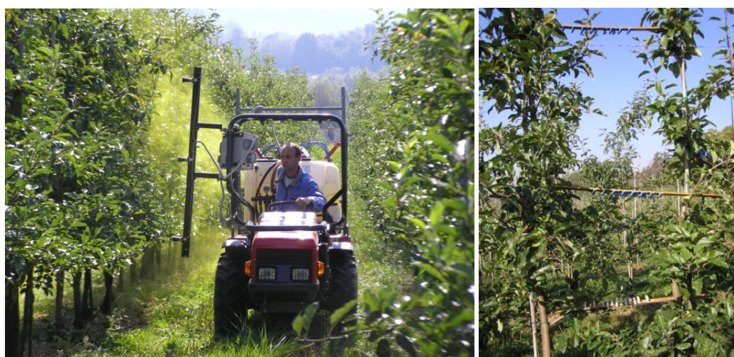
Figure 6. A prototype sprayer during the experiment in the orchard (left), detail with measuring positions on the tree (right).
