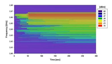
Once the interference levels have been characterized, the performance of the radiolinks between wireless sensors can be analyzed, in the same scenario previously described. The RF modules employed have been Digi XBee Pro models, which can operate using channels 12 to 23 of the IEEE 802.15.4 standard.
