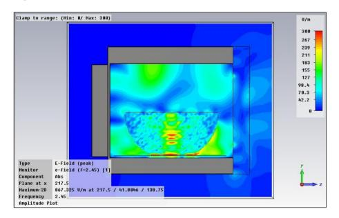
The electromagnetic field distribution calculated outside the oven is necessary for the later 3D ray launching simulations, which will allow the estimation of interference effect within the complete simulation scenario and will be described in the following section.
