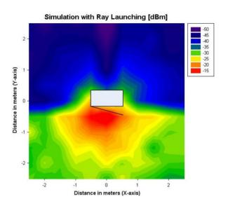
**Figure 8.** 3D Ray launching results for a height of 0.7 m with the losses calibration in the back plane of the microwave. (a) Bidimensional plane. (b) Tridimensional plane.
