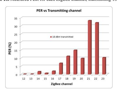
Figure 16. Measured PER for each ZigBee channel, transmitting 18 dBm.
