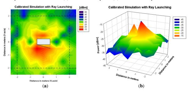
To overcome this issue, a calibrated equivalent simulation antenna has been computed from the measurements of the back plane of the scenario. By using the Friis formula and normalizing by the number of launched rays, the calibrated transmitted power has been calculated. Ray launching simulation has been performed again for the back plane with the new calibrated antenna. Figure 8
