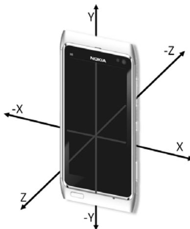
Figure 1. The smartphone body frame defined for the Nokia N8 consists of three axes and six directions, and it uses the right-hand Cartesian coordinate system. The various sensors all use the common body frame.
