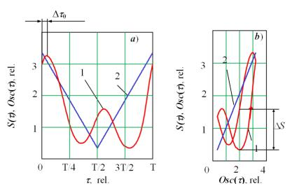
The signal shift  $\Delta \tau_0$  ( $\Delta S$ ) is more obvious in under-focused and over-focused modes and is zero in sharp focusing regime (Figure 7). If we compare their relationship, we see an increase of the second harmonica on transition to the over-focused modes. We see that under an under-focused regime, the beam interacts with a forward wall and the bottom of the keyhole; whereas, under an over-focused regime, it interacts with the forward and rear walls almost equally.
