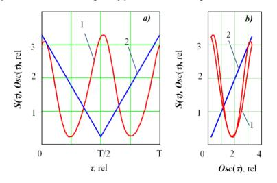
Figure 6 presents the results for oscillation along the joint. The asymmetry of the figure reflects the asymmetry of the keyhole in the longitudinal direction. In the spectrum of a secondary signal in this case, the first harmonic of the signal prevails. The lag (shift) of the secondary signal relative to the current of the deflection coils can be noted ( $\Delta \tau_0$  or  $\Delta S$ ).
