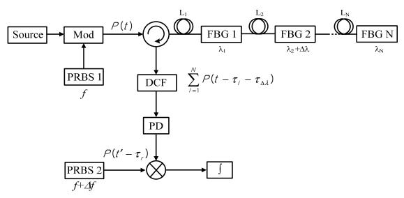
Mod: modulator, FBG: fiber Bragg grating, DCF: dispersion compensation fiber (wavelength to time conversion module), PRBS: pseudo random binary sequence, PD: photodetector
