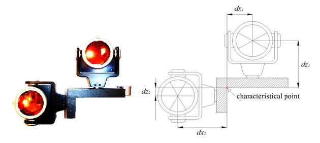
The position of the characteristical point, representing the upper inner edge of the rail, can be derived from the measured positions of both precise prisms. Accurate dimensions of the platform need to be known, *i.e.*, offset of both prisms from the edge of the rail.
