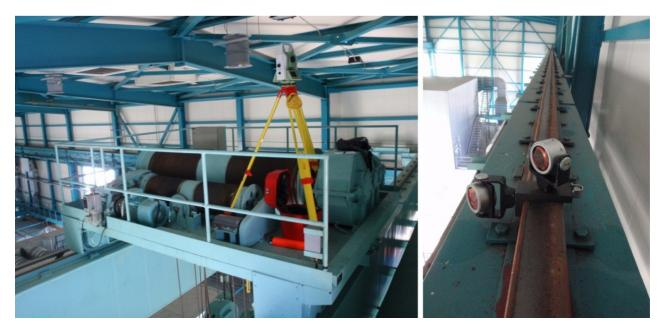
The positions of both prisms were measured twice using the ATR function, which provides homogenous sighting precision for each measuring point on the rail. The platform was placed on each rail 38 times. For each stabilization of the platform each prism was measured twice. As a result we got 304 measured points with the polar coordinates [s, z, d].
