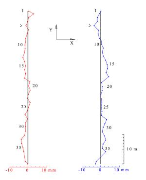
3.4.2. Elevation Differences of Crane Rails
