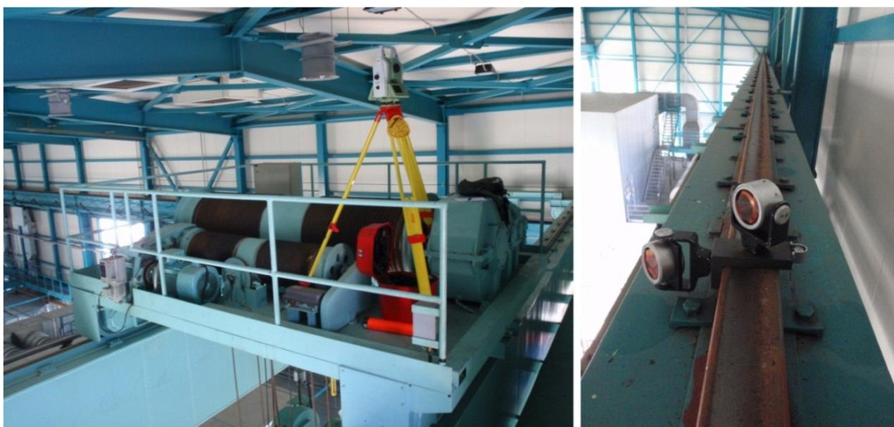
The positions of both prisms were measured twice using the ATR function, which provides homogenous sighting precision for each measuring point on the rail. The platform was placed on each rail 38 times. For each stabilization of the platform each prism was measured twice. As a result we got 304 measured points with the polar coordinates  $[s, z, d]$ .
