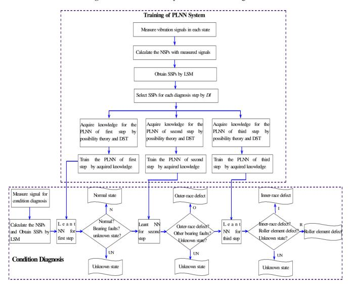
Figure 6. Flowchart of sequential condition diagnosis.
