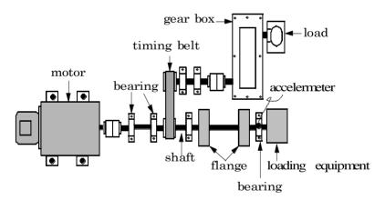
Figure 2. Experimental setup for rolling bearing fault diagnosis.
