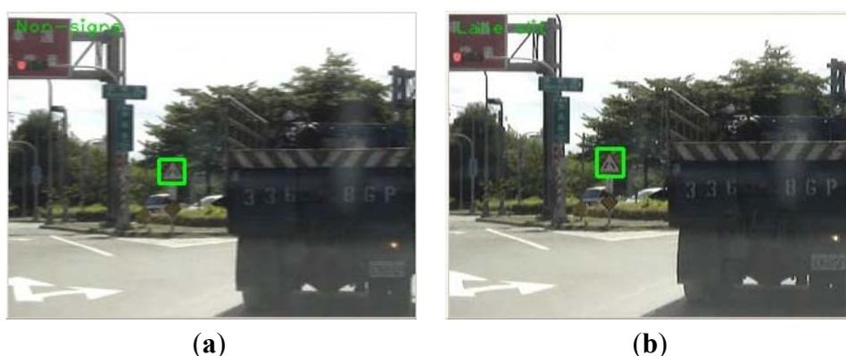
Figure 14 shows some example frames in a sequence. According to the detecting area setting, Figure 14(a) shows the case that the road sign is in the detecting area but too small to detect. The road sign in Figure 14(b,c) can be detected and correctly recognized. Figure 14(d) shows the target is out of the detection area, and thus the system cannot detect it.
