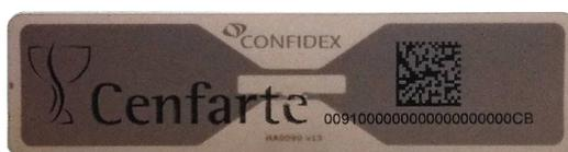
The tag works using EPC Gen2 Class1 protocol, its frequency range is from 860–960 MHz and its reading range is from 4 to 6 m, enough for a wagon van. The price of tags is decreasing year by year,
