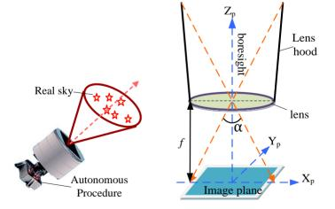
According to the coordinates of star points in the focal plane coordinate system  $X_p$ - $Y_p$ , it is easy to obtain the coordinates matrix S of star points in the star sensor coordinate system  $X_s$ - $Y_s$ - $Z_s$ . Combined with stars coordinates G in the inertial coordinate system  $X_L$ - $Y_L$ - $Z_L$ , the attitude A can be determined as the form of 3 × 3 direct cosine matrix by:
