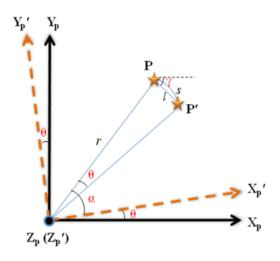
where  $X_p \cdot Y_p$  is the coordinate system of focal plane,  $X_p' \cdot Y_p'$  is the corresponding coordinate of  $X_p \cdot Y_p$  after rotation, and  $\theta = w_z t$ , where *t* is the rotation time in *T*. The star point *P* shifts to *P'* along the circular arc *s* with radius *r* in the focal plane. It is reasonable to assume that the rotation axis and the motion parameters are constants, and *l* is approximate to *s*. As a result *l* can be expressed as:
