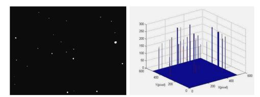
Figure 7. Star image and its gray distribution after discarding singularity spot.
