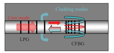
Figure 1. Schematic diagram of hybrid LPG/CFBG refractometer.
