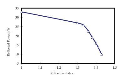
Figure 5. Reflected power of hybrid LPG/CFBG versus RI.
