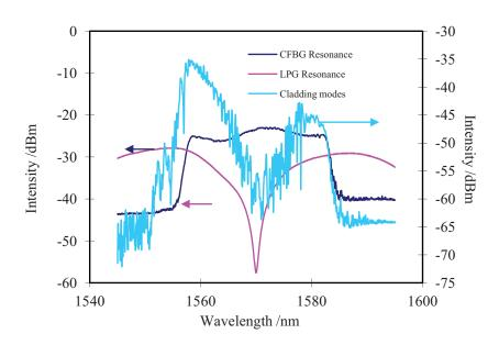
Figure 2. Spectra of LPG and CFBG before and after splicing.
