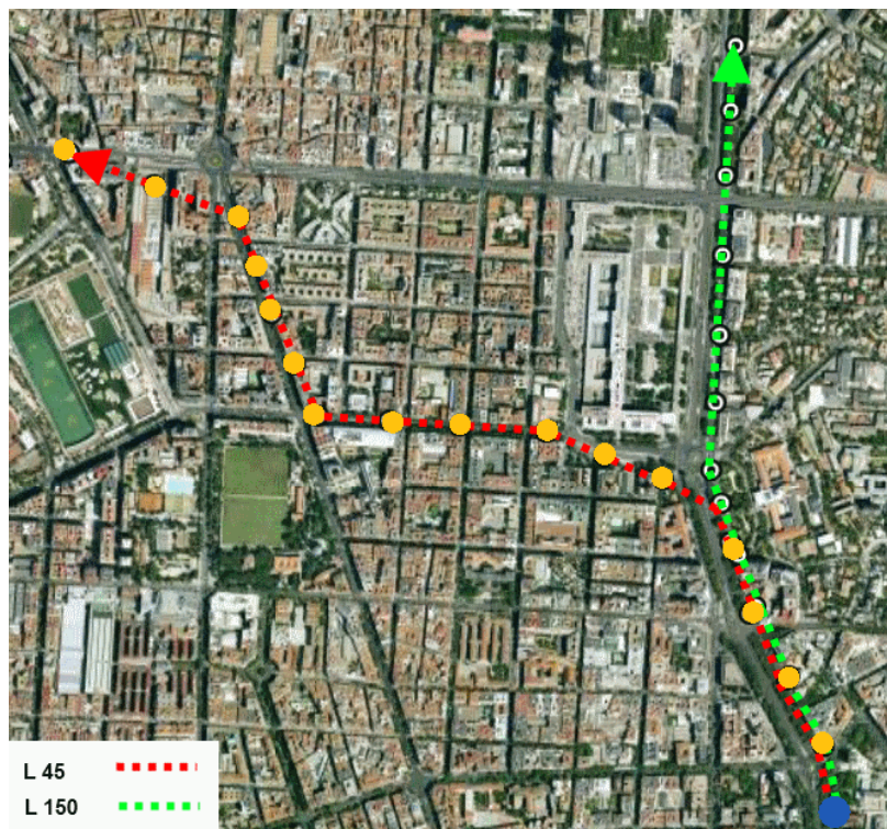
Figure 14. Test scenario. Paths marked in red and green are the bus lines considered. Blue point is the starting location of the user. Yellow dots are the places where the terminal switches from one cell to another and makes the prediction about the next location.
