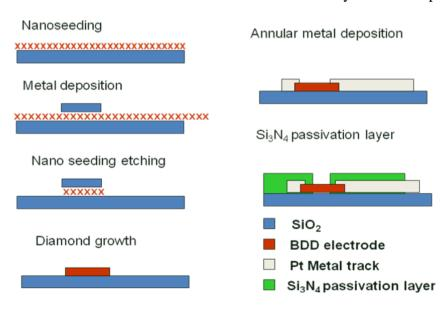
Figure 1. Schematics of diamond ultramicroelectrode array fabrication process.
