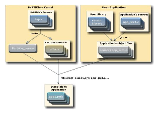
Figure 5. Building Process of Sensor Application.
