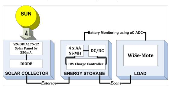
Figure 1. Model for a solar powered system.
