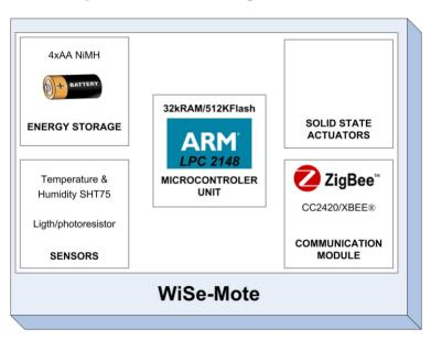
Figure 2. Model of the Open-WiSe mote.
