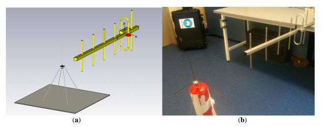
The antennas are operating in the near field, so equations for far field path loss cannot be used to determine the RF power level that can be received by the leaf-node antennas, and would also ignore the effect that mutual coupling will have on the power transfer. Instead, the antenna arrangement was modeled using CST Microwave Studio and a two-ray propagation model [15,16].
