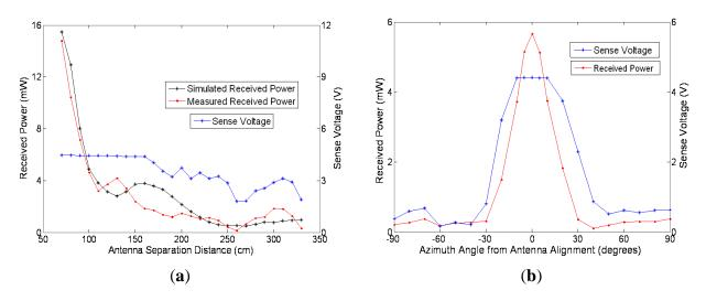
Figure 6(b) shows the measured received RF power and sense voltage at a separation distance of 1m while the antenna scans from  $-90^{\circ}$  to  $90^{\circ}$  with the leaf node located at zero degrees. This plot verifies the use of the sense voltage to determine the alignment of the leaf node and the base transmitter. Comparatively to Figure 6(a), it can be noticed the peak of the sense voltage levels off as it meets the condition described in Equation (1).
