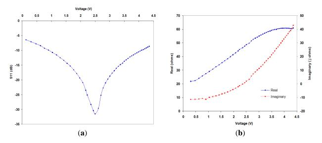
**Figure 7.** (a) change of S11 as supercapacitor charges at 6 dBm; (b) Impedance change as supercapacitor charges.
