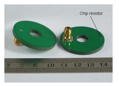
Figure 6. Photograph of the fabricated antenna.
