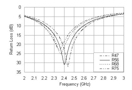
Figure 5. Simulated return loss curves with different values of *R*.
