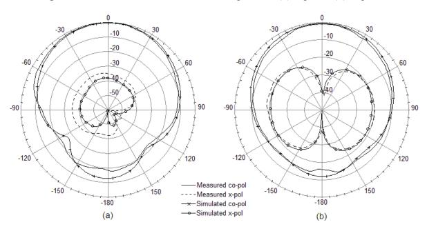
Figure 8. Measured and simulated radiation patterns. (a) E-plane. (b) H-plane.
