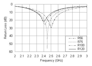
Figure 10. Measured and simulated return loss curves of the antenna along with the installation base.
