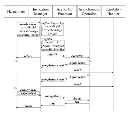
Figure 5. Interaction diagram of asynchronous invocation.
