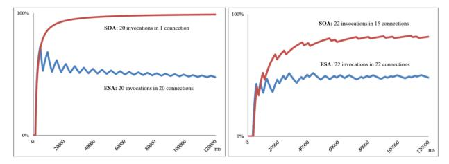
Figure 11. Average resource utilization for Bluetooth in Case #1 (left) and Case #2 (right).
