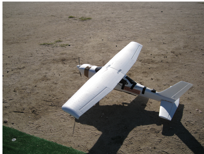
Figure 1. Mentor Multiplex aircraft modified by the authors to be a UAV.
