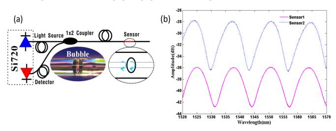
The air bubble was realized by adjusting the splicing parameters of the commercial arc splicer (Fitel S176) to certain values. Figure 5(b) shows the reflective spectra of such two air-bubble-based FPIs with cavity length of approximately 91  $\mu$ m, and the high-quality interference spectra with a fringe visibility of ~8 dB were observed. Both the influences of strain and temperature on the reflective interference signal
