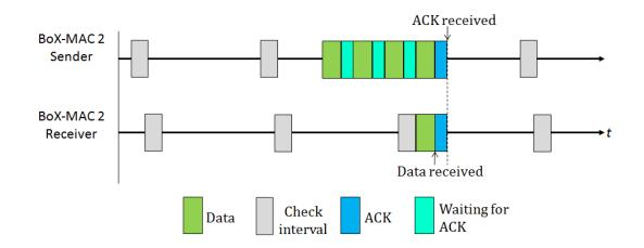
Although BoX-MAC reduces the energy consumption by 30% to 50% compared to other existing approaches, the latencies and the channel contention along a path increase linearly with the number of nodes on the path. In this work we investigate the impact of the network delays on the energy consumption and throughput in BoX-MAC-2.
