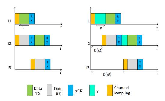
As indicated, CLAC uses  $\gamma(i_k)$  to express the delay experienced by a packet at the node  $i_k$ . This value is specific to each node and it depends on several factors: the network topology, the duty cycle, the frequency with which the application generates traffic, *etc*. We have analytically computed the value of  $\gamma$  by analyzing two different multi-hop scenarios: a linear and a tree-based data collection topologies.
