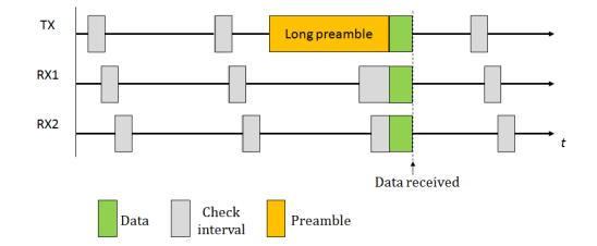
Figure 1. Basic preamble sampling scheme.
