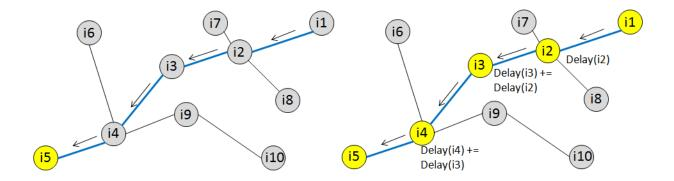
Figure 3 shows, on the left hand side, a simple scenario where  $i_1$  sends data to a remote receiver  $i_5$ . The arrows show the path between the two nodes as computed by CTP. The right hand side shows the delays incurred as data propagates from  $i_1$  to  $i_5$ , and how these are accumulated during the multi-hop transmission.
