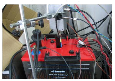
Figure 5. QCM sensor placed inside the battery during real time measurements.
