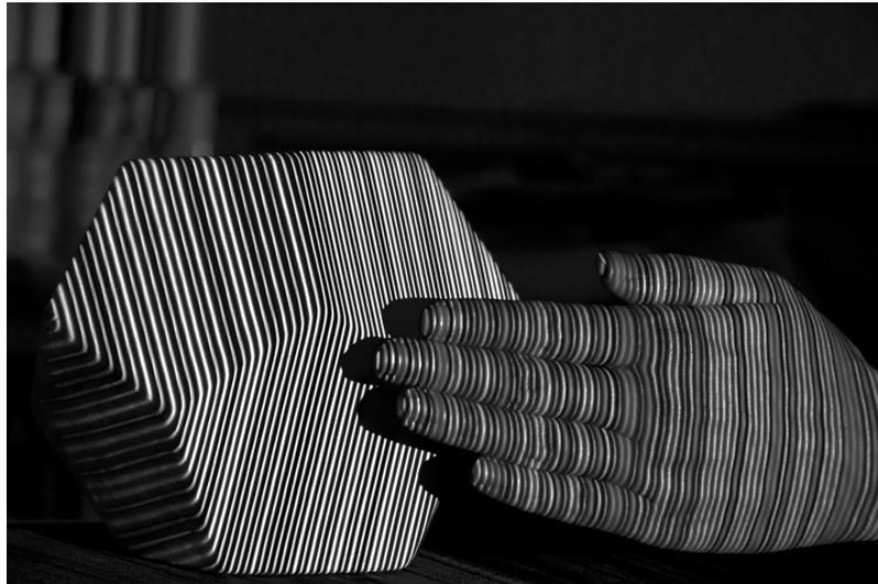
Figure 3. Reconstruction examples: (a) hand; (c) face and (e) hand with background of hexahedron under the pattern illumination. Reconstructed surface of the (b) hand; (d) face and (f) hand with background of hexahedron.
