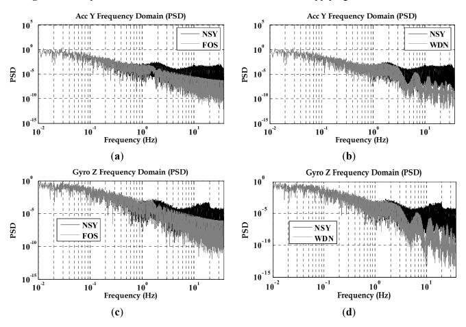
Figure 7. PSD plots for TG6000 inertial sensors before and after applying both FOS and WDN.
