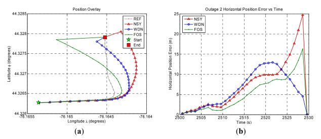
**Figure 10.** Land vehicle experiment position domain results for GPS outage 3. (**a**) Position domain plot. (**b**) Horizontal position error plot.
