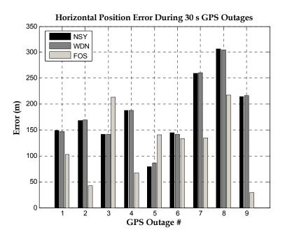
Figure 14. Positioning accuracy at the end of 9 GPS outages for MEMS IMU for the 2nd road test.
