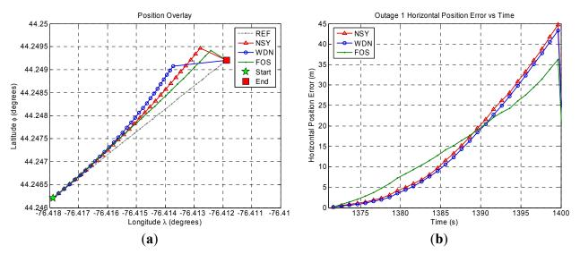
**Figure 9.** Land vehicle experiment position domain results for GPS outage 2. (**a**) Position domain plot. (**b**) Horizontal position error plot.
