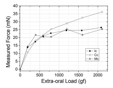
From the orthodontic forces (fixed appliance) and orthopedic forces (extra-oral appliance) it was possible to observe response on teeth roots between 0 and 35 mN. On the other hand no tensions from orthodontics and orthopedics forces were detected at the surface of the maxilla model by the FGB a, b, c and d sensors (Table 4).
