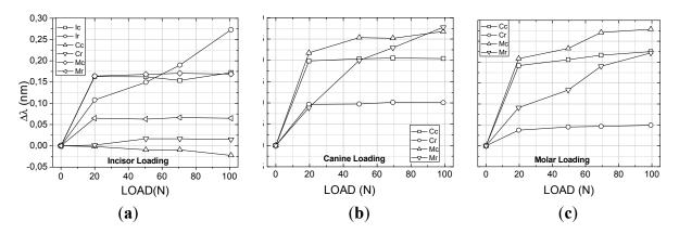
The multiplexed fiber sensors FBG a, b, c and d did not experience any deformation which means that probably the tensions were not transferred to the surface of the material representing the maxillary material bone. Table 2 summarizes the final wavelength shift experienced by the gratings.
