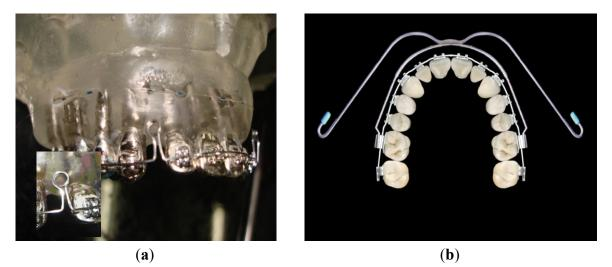
The measurements with the orthodontic appliance were repeated three times for each tooth: incisor, canine and molar, all of them at the left side of the maxilla model. The loading procedure followed the mechanical test changing only the range of the forces from 0 to 2,600 gf (25.49 N).
