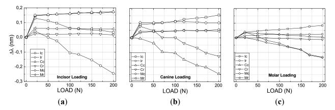
Figure 4 shows the results of all six sensors placed at the teeth, both at the crown and apex, for vertical loading of the incisor, canine and molar teeth. As expected all teeth that are directly receiving the applied loading sense compressive forces both at the root, near to the crown, and at the apex. It is observed however that for small loads either the apex or the root might have an inverse behavior which
