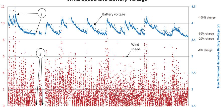
Figure 8. Tree powered sensor node battery voltage and wind speed; representative sample, February to May 2011.
