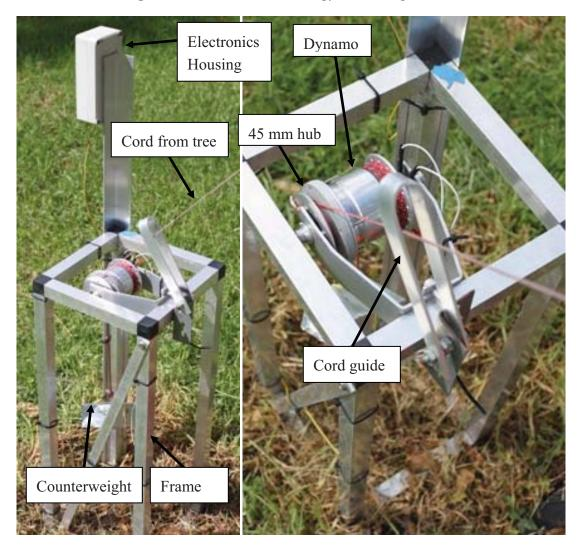
Figure 1. Tree movement energy harvesting device.
