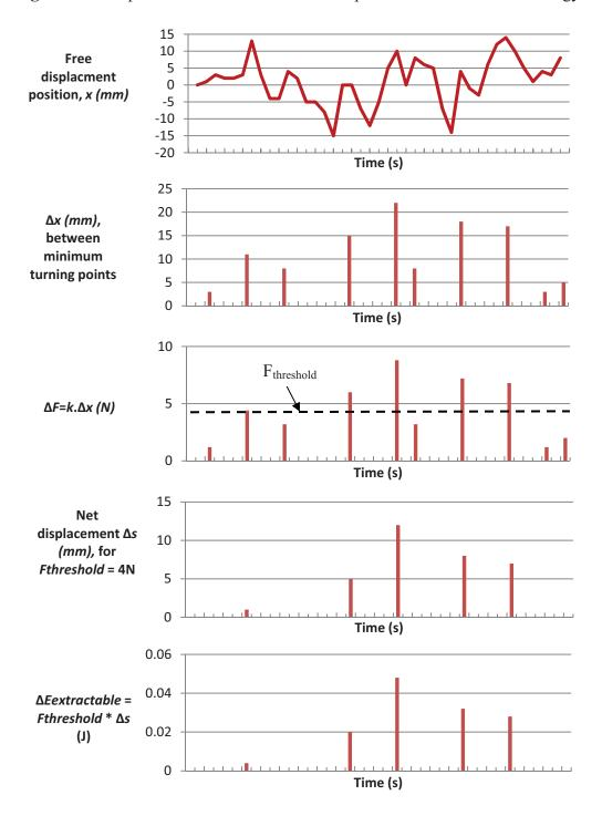
Figure 3. Example transformation from free displacement to extractable energy.
