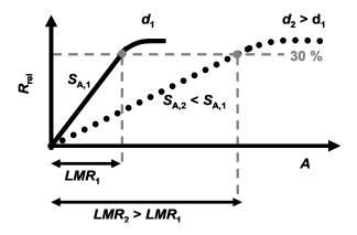
However, like the base resistance, the sensitivity to  $NO_x$  is inversely proportional to the film thickness d. This agrees with a simple model concerning nitrate formation at the surface of the sensitive layer. It was demonstrated that  $NO_x$  can be detected linearly until the sensor resistances
