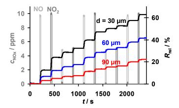
A more detailed analysis of the dependency of the sensitivity, the linear measurement range and the sensor response time on the thickness of the sensitive layer is given in the next sections.
